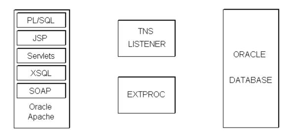
Communication between the web server and the database server is first channelled through the Listener. This Listener is responsible for setting up connections to the oracle database instance and once joined the listener steps out of the picture. As we shall see further into this paper the Listener does have more to do than just this. The Listener plays a key role in executing external procedures for the database server.
